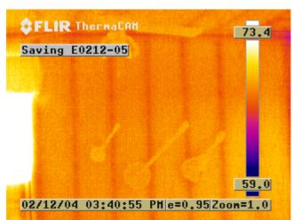
This Infrared image shows a well insulated wall.
